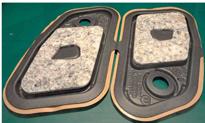
Figure 29 Adhesive foam for door water shield with excellent acoustic insulation
