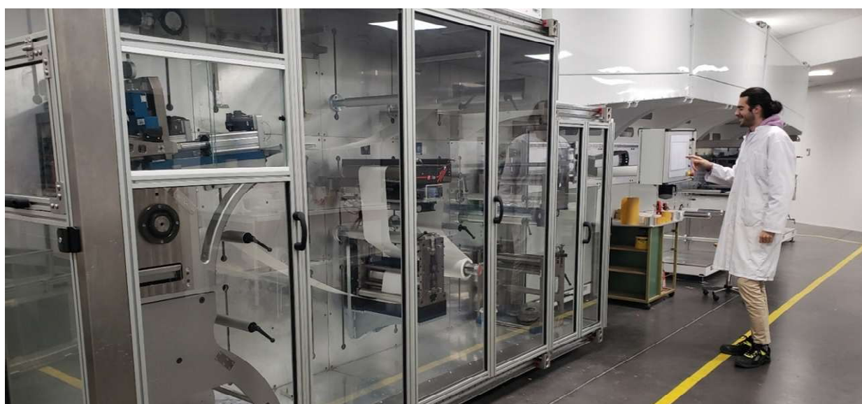
Figure 25 Our industrial scaled pilot line dedicated to the development of innovative and sustainable pressure sensitive adhesives
