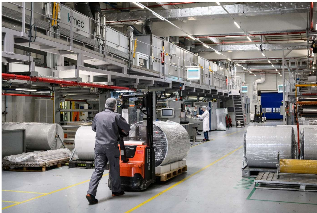
Figure 13 the SuperKMEC coating line of Chenôve plant after the 20 m extension transformation
